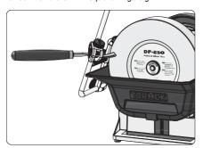
Example shows sharpening a flat bevel on a V-tool with the SVS-38 Short Tool Jig.
