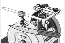
Example shows sharpening a flat bevel on a knife with the KJ-45 Centering Knife Jig.
