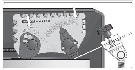
Use the top angle scale, marked with MB-100/MB-102.
