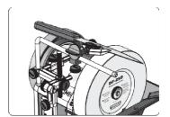
Sharpening knives edge trailing using the KJ-45 Centering Knife Jig. You set the angle the same way you would normally do, either with the WM-200 Angle Master or the Tormek Marker method.
