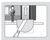
**Tip** The jig is made with a large supporting surface for good control even when grinding long tools. For short tools, you can trim the jig surface as necessary to clear the handle.
